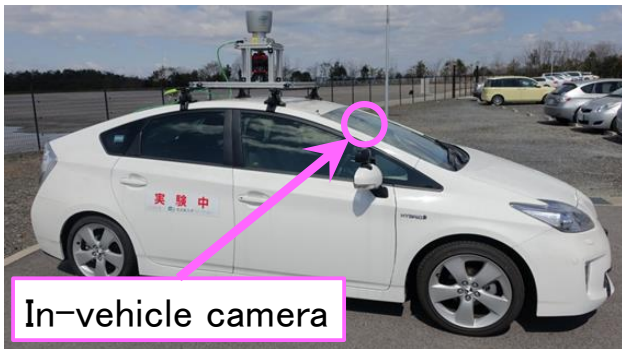
Fig.4 Installing position of the in-vehicle camera.
