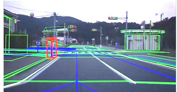
a) LiDAR Based Moving Object Detection Result & Overlapped Vector Map
