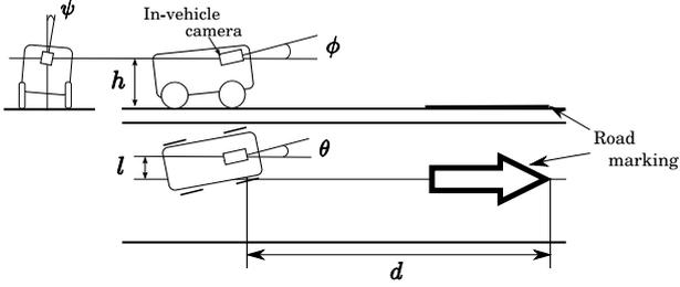
Figure 2: Geometrical position and parameters.
